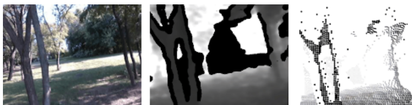
Figure 4. Outdoor stereo vision in a simple park environment produced reliable depth only at short range, leaving distant regions sparse, noisy, or invalid in the 3D point cloud.
