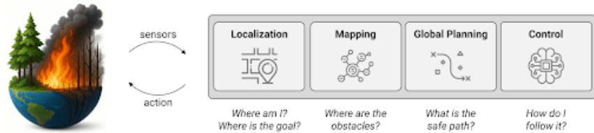
Figure 1. Simplified view of the autonomy pipeline used in many drone systems. To navigate safely, the vehicle must estimate its position, interpret its surroundings, plan a safe path, and control its motion. In disaster environments, uncertainty in any one of these stages can propagate through the system and reduce overall performance.
