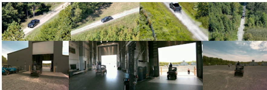
Figure 3. Perception degradation during autonomous flight. (a) Dust from a pickup truck reduced visibility and introduced visual artifacts during vehicle tracking. (b) Abrupt illumination change during an indoor-to-outdoor transition saturated the camera image and reduced usable visual information.
