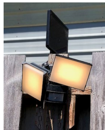
Figure 23: Solar Motion Detection Lights on Fence by a Cache Photo courtesy of Susan Graves
