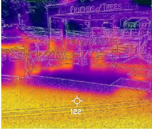
Figure 27. Image taken with a Forward Looking Infrared (FLIR) camera at SE 7 th Ave & Sandy Blvd. July 28, 2023, 2:09 PM. Surface temperature of the pavement outside the awning is 122 degrees F.
